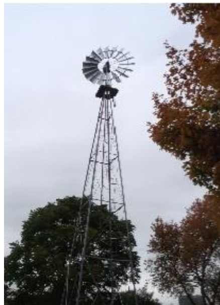
A genuine Aermotor windmill installed by Amish workers from Ohio now graces the grounds at the Queens County Farm Museum.
